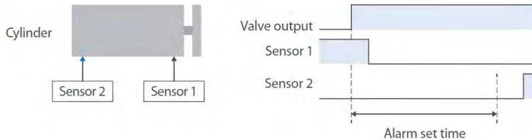
The basic method for monitoring a pneumatic actuator is to measure the cycle time for the extension and retraction of the cylinder. **Monitoring this time can identify immediate performance issues and by tracking this value over time can reveal a slowly degrading performance.**
