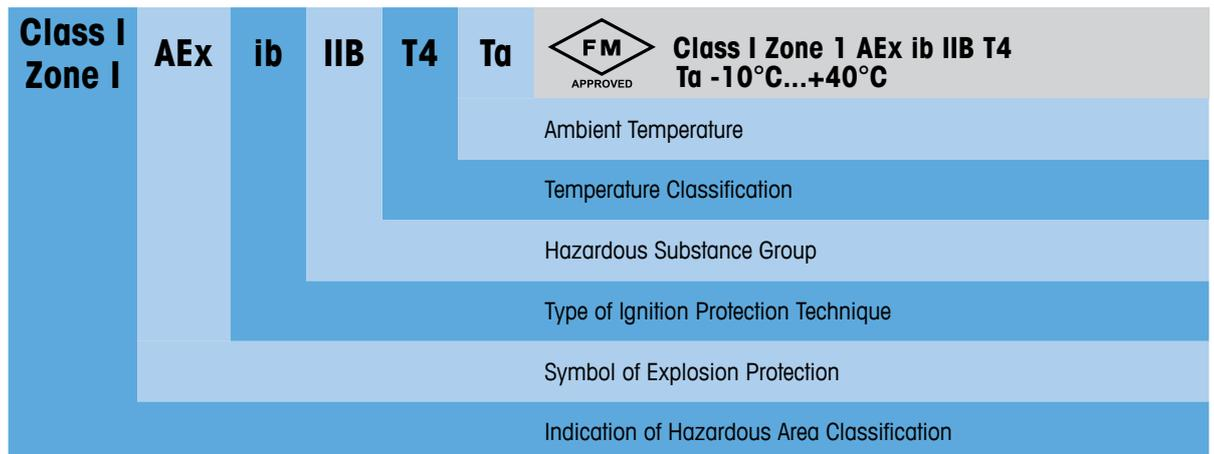
Figure 9. Example of the Electrical Equipment Marking According to NEC 505.
