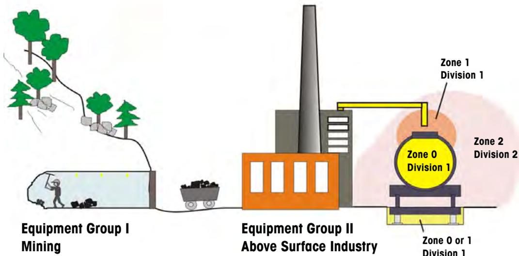
Figure 4. Definition of Equipment Groups and Categories According to the ATEX94/9/EC
