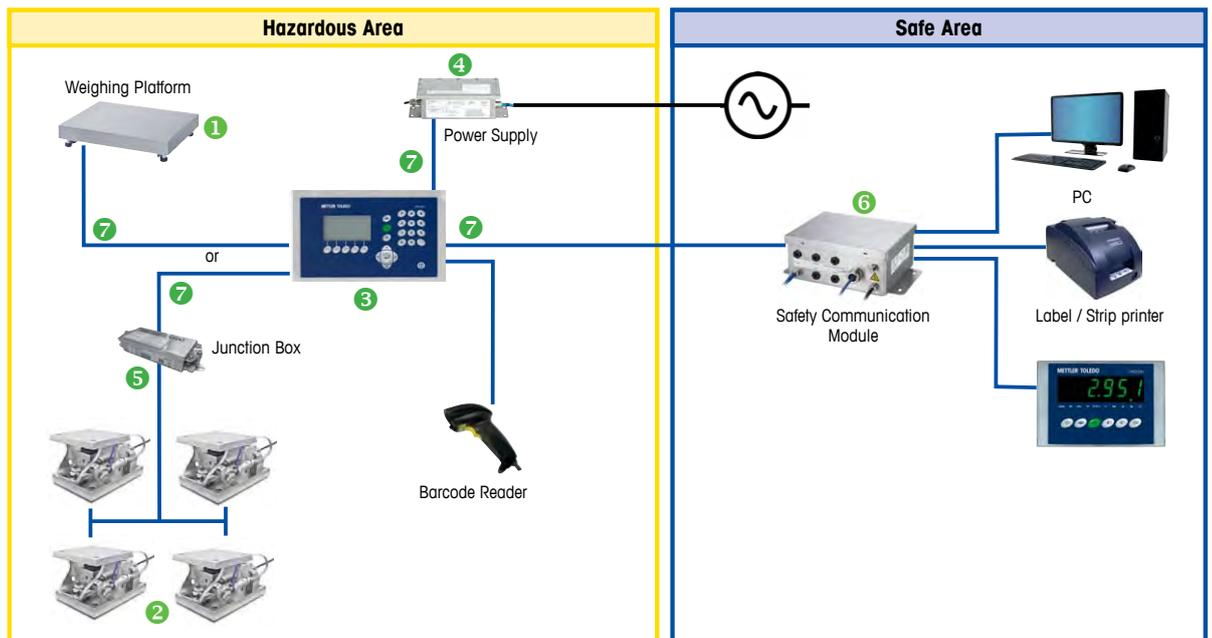
Figure 10. Weighing System Configuration in Hazardous Area Zone 1 / 21, Division 1
