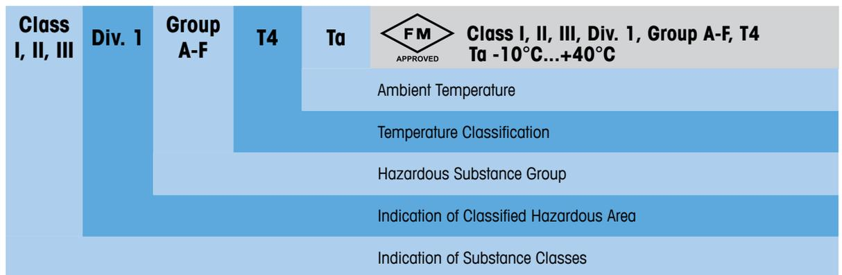
Figure 8. Example of the Electrical Equipment Marking According to NEC 500.
