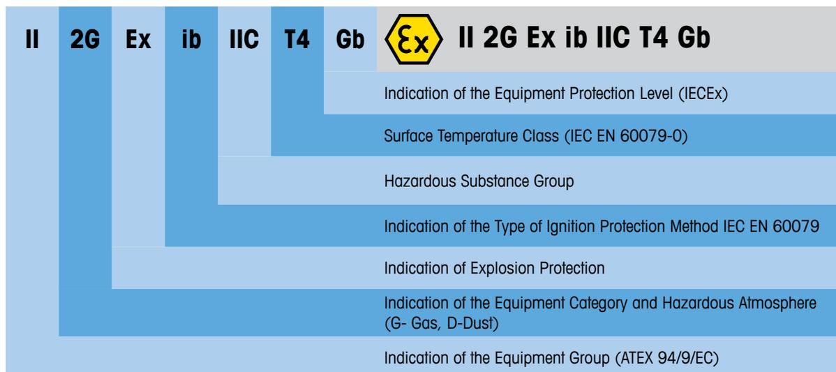
Figure 5. Typical Electrical Equipment Marking According to ATEX 94/9/EC
